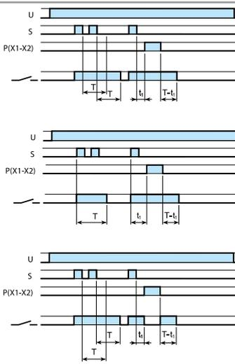
**(BEp) Off-delay with control signal and pause signal.**
