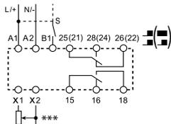
\*\*\* Regulated using an external potentiometer (10 kΩ - 0.25 W).
